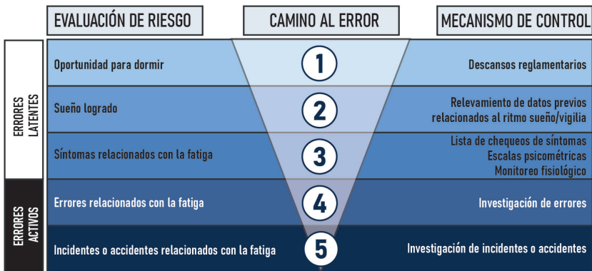
Figura 9. Modelo de un sistema de gestión de riesgo de fatiga. Adaptada de Dawson (2012). Fatigue-proofing: A New Approach to Reducing Fatigue-related Risk Using the Principles of Error Management.
